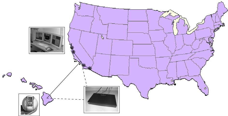
Figure 1. Schematic representation of the Keck remote observing network. The asterisks denote the four remote observing stations currently operational or under development. The dotted line denotes the backup network link via a group of ISDN lines.
