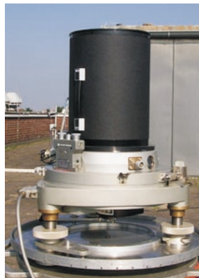
Figure 1. The digital zenith camera TZK2-D
