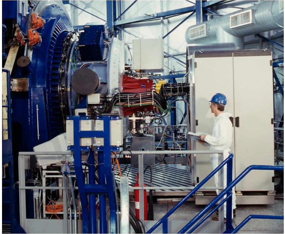
Figure 1. NAOS-CONICA on the Nasmyth B focus of Yepun. From left to right, one can identify the Nasmyth B rotator (dark blue), NAOS (light blue), the back-end of NAOS (white), CONICA (red) and the cables that transport coolant, power and signals between NAOS-CONICA and the co-rotator.
